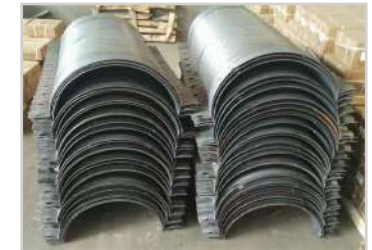
flanged nestable CSP segments
