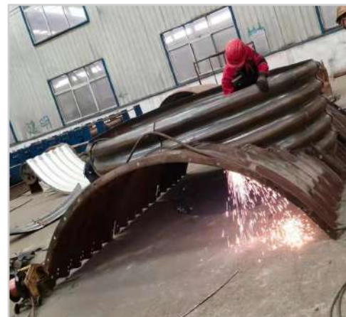
Structural Plate Tee in Shop
